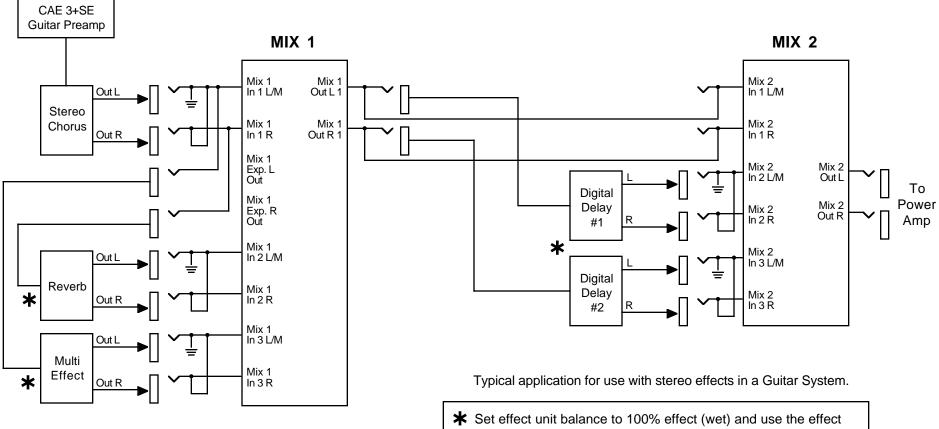
units output level for balance between "effected" sound and dry (unprocessed) sound. The dry (unprocessed) sound passes through inputs 1 on both mixers.
